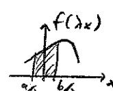
$$\int_a^b dx f(x) = \lambda \int_{a/\lambda}^{b/\lambda} dx f(\lambda x) \quad (\text{also } x \rightarrow \lambda x, dx \rightarrow \lambda dx \text{ Grenzen} \rightarrow \text{Grenzen } / \lambda)$$
