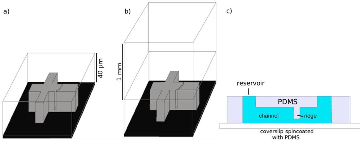
**Fig.3:** Scheme of double-layer soft lithography. a) First layer of h-PDMS  $40\ \mu\text{m}$  in height (not to scale), to stably mold the nanoslit. b) Second layer of PDMS  $1\ \text{mm}$  (not to scale), for better handability. c) Cross section of assembled chip with reservoirs and running buffer (blue).
