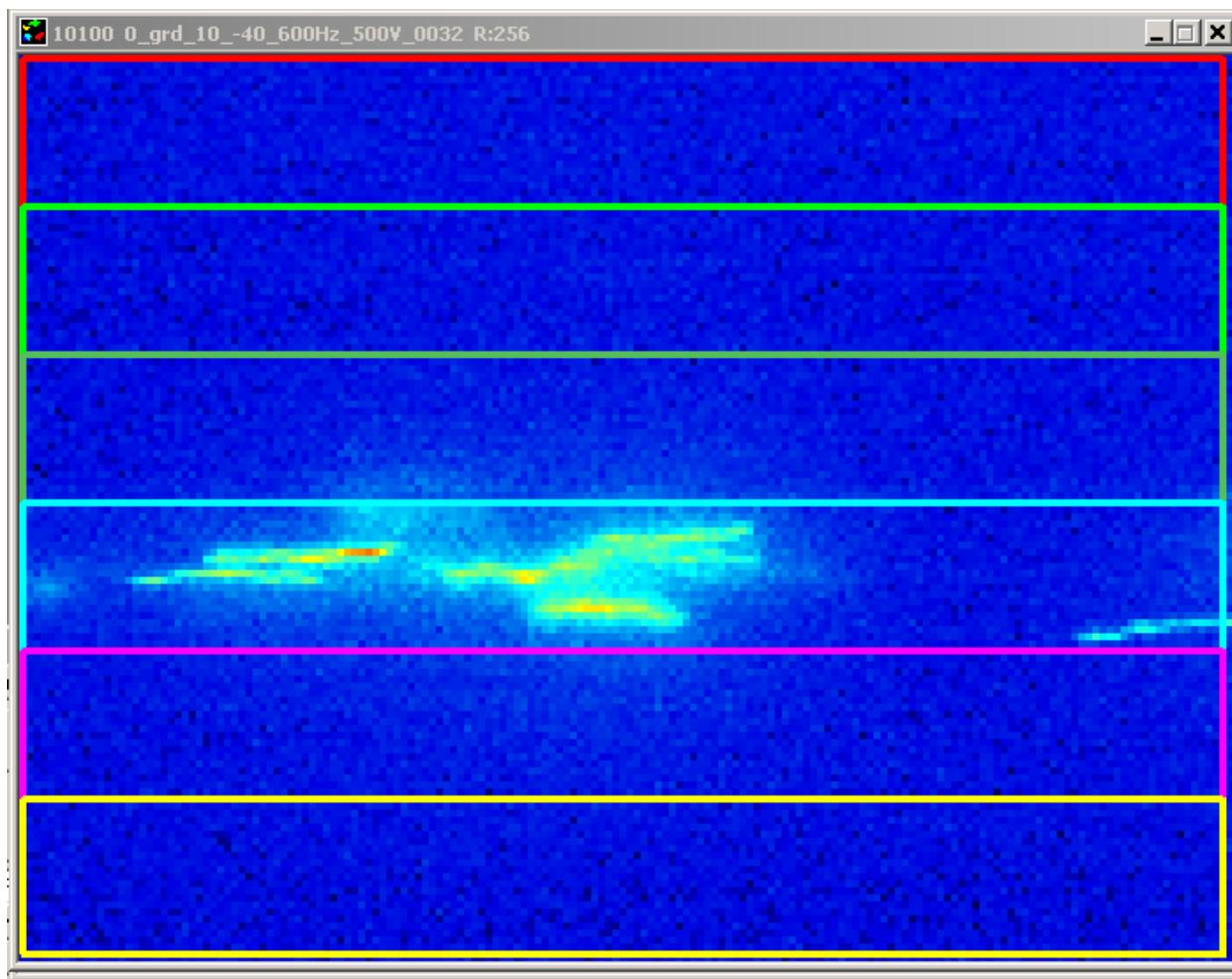
**Fig.5:** The region of interest is partitioned in six slices, each with height of 11  $\mu\text{m}$ . To determine the analytes distribution the fluorescence intensity is measured in each slice separately, along the scanning procedure, and averaged over up to six overlapping slices.
