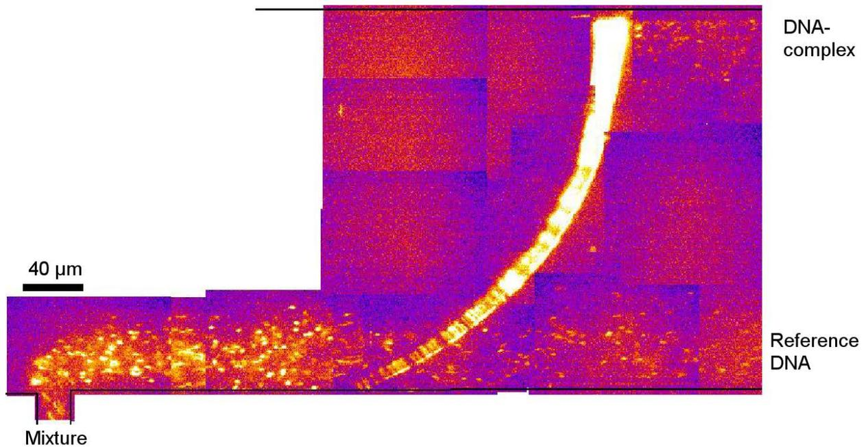
**Fig.4:** Detection of complex-formation and separation. Fluorescence images (collage) at the nanoslit. From the left, a mixture of DNA is continuously injected (yellow spots correspond to single DNA molecules). The reference DNA passes the nanoslit unhindered, whereas the DNA-complexes are trapped on the ridge and migrate towards the opposite channel side before they escape due to Brownian motion. Evaluation of the separation resolutions reveals a clearly baseline-separated resolution.
