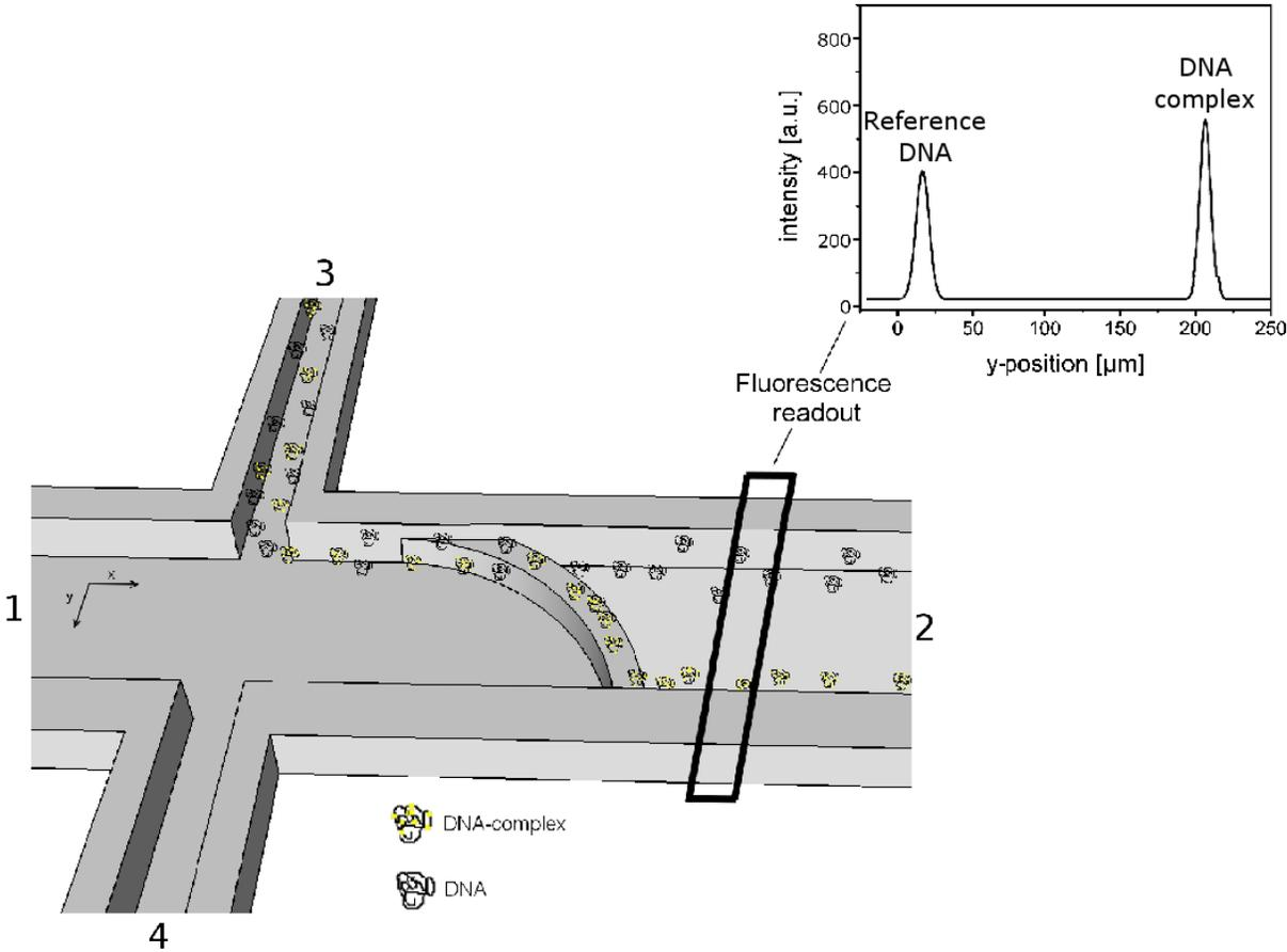
**Fig.1:** Scheme of the continuous-flow separation and analysis. The analyte is injected towards the ridge as a narrow stream. At the ridge, one species is deflected; the second species passes the ridge unaffected. Downstream of the ridge the response is monitored by fluorescence intensity distributions.
