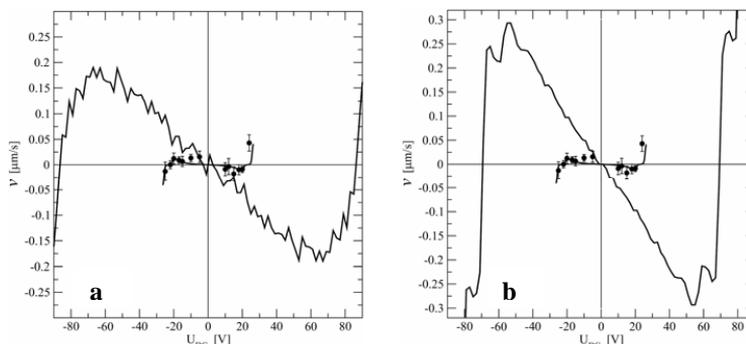
Fig. 2: Numerical simulation of particle velocity for  $1.9 \mu\text{m}$  sized particles versus applied static offset force  $U_{DC}$ . a) Simulation for the design demonstrated in fig. 1a. For comparison, recently published [1] experimental data with numerical simulations are shown around the origin in both a) and b) (dots with line around the origin). b) Simulation for the design demonstrated in fig. 1b
