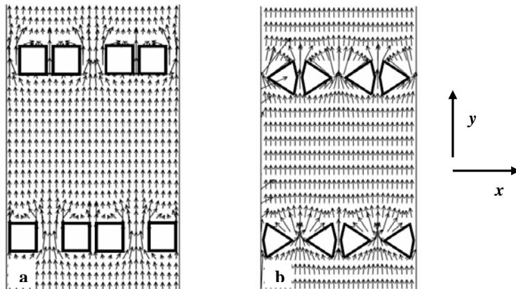
Fig. 1: Section of microstructured post array designs for ANM in a microchannel with simulated force field (arrows): a) Square posts and b) sharpened posts.
