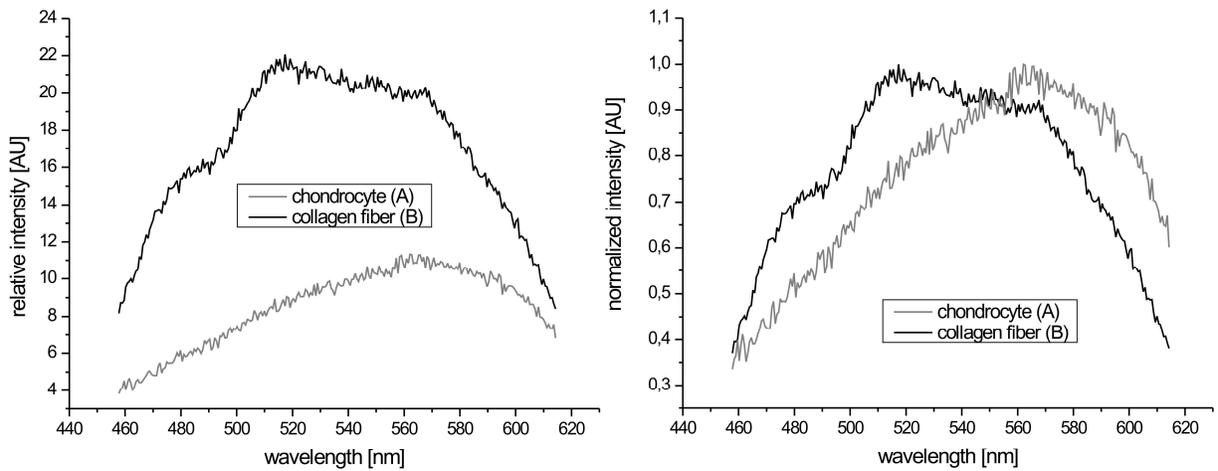
Figure 6: Emission spectra of I/III collagen fibers and chondrocytes on sponge-like membranes after 2-photon excitation (32 foci à 5.5 mW, 785 nm, 650 ms exposure time), prism based home build spectrometer with  $\pm 7$  nm wavelength accuracy, spectra taken from regions in Fig.7 which clearly could be identified as collagen fiber and as chondrocyte, left: relative intensity, right: normalized intensity.
