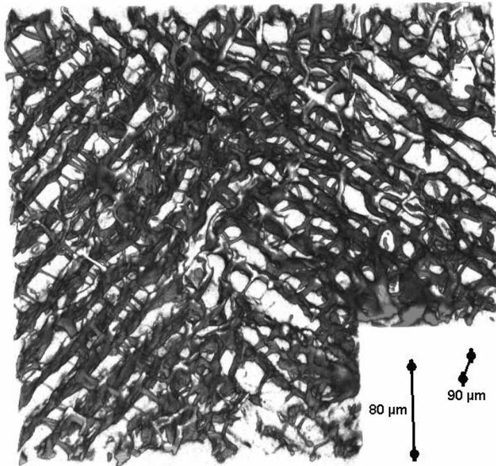
Figure 5: Digital reconstruction based on native 2-photon induced (820 nm, PMT detection) fluorescence, no emission filter, dataset contains images of up to 90 μm inside the sample
