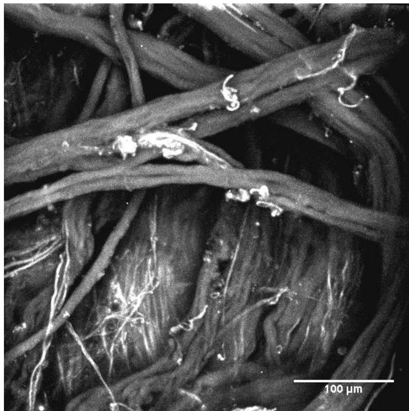
Figure 3: I/III-collagen fleece membrane, 2-photon (810 nm, 64 foci à 4.4 mW, 1 s exposure time) excited native fluorescence, Filter: HQ575/50, maximum intensity projection of 240 optical sections à 1  $\mu\text{m}$ .
