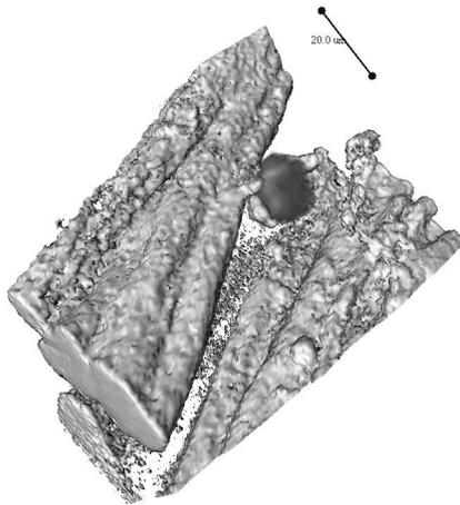
Figure 4: Digital reconstruction based on 2-photon induced (820 nm, single focus < 15 mW, PMT detection) native fluorescence (HQ 525/50 and HQ 575/50 emission filters) and SHG (HQ 410/20 emission filter), scale bar represents 20 μm.
