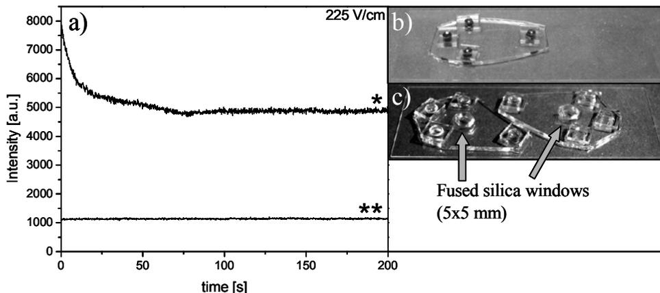
Figure 2. Fluorescence background reduction: (a) Fluorescence background of the microchannels filled with separation buffer (100 mM TRIS, 100 mM CHES, 4 % Pullulan, pH = 11,0), with 1000  $\mu\text{m}$  pinhole and 500  $\mu\text{W}$  laser power,  $\lambda_{\text{ex}} = 266 \text{ nm}$ , (\*) within the PDMS-chip and (\*\*) within a PQW-chip. (b) Photograph of a PDMS-chip and c) two PQW-chips.
