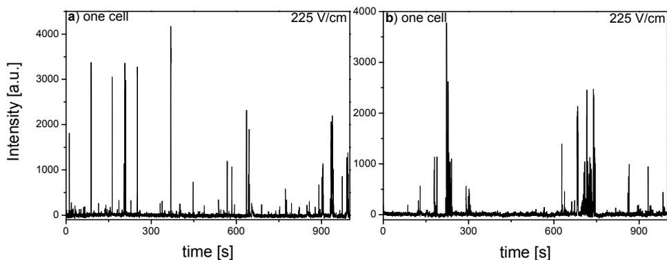
Figure 4. (a) Baseline corrected electropherogram from a single Sf9 cell with native UV-LIF detection ( $\lambda_{\text{ex}} = 266 \text{ nm}$ ). Separation buffer (100 mM TRIS, 100 mM CHES, 4 % Pullulan, pH = 11,0), 1000  $\mu\text{m}$  pinhole and 500  $\mu\text{W}$  laser power. The cells were electrically lysed with an electric field pulse (1800 V/cm, 50 ms). The channels in the PQW-chip were coated with F108. (b) Electropherogram of a single Sf9 cell with equal conditions as in (a).
