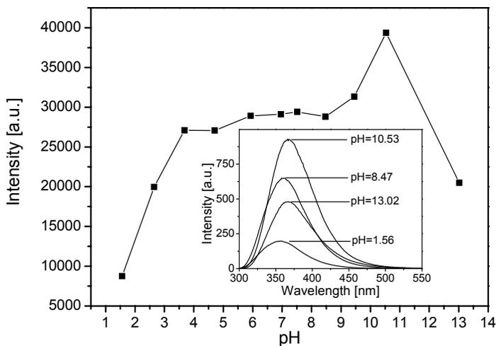
Figure 3. Increased signal intensity at basic pH: dependence of fluorescence intensity on pH for 10 mM tryptophan (Trp) solutions (in PBS), ( $\lambda_{\text{ex}} = 280 \text{ nm}$ ,  $\lambda_{\text{det}} = 335\text{-}385 \text{ nm}$ ). Inset: Selected emission spectra of the same Trp solutions from pH 1.6 to 13.0 ( $\lambda_{\text{ex}} = 280 \text{ nm}$ ).
