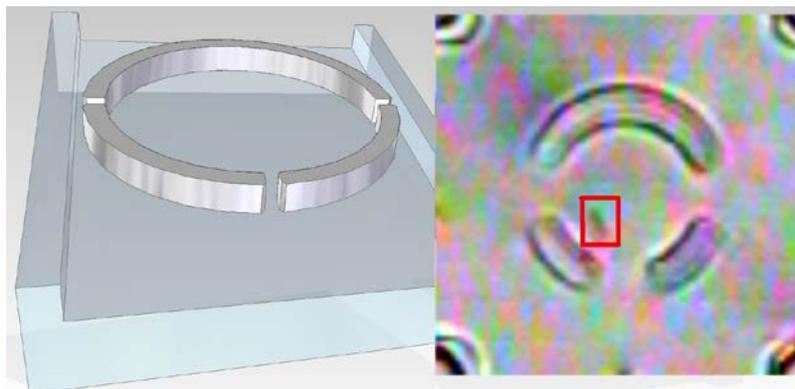
Figure 2: Trapping feature for the *E. coli*. Left) sketch of the feature. Right) microscopy image of a single *E. coli*, marked with the red square, in the trapping feature. In the corners of the picture the corners of the channel is visible to indicate the dimension; the channel width was 30 μm, the channel height was 6 μm.
