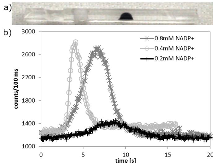
Figure 1: Cofactor detection by UV/VIS spectroscopy. a) Cross-section of chip with black-PDMS spot at detection point. b) Fluorescence intensity for pinched injection of NADP<sup>+</sup> at varying concentrations.
