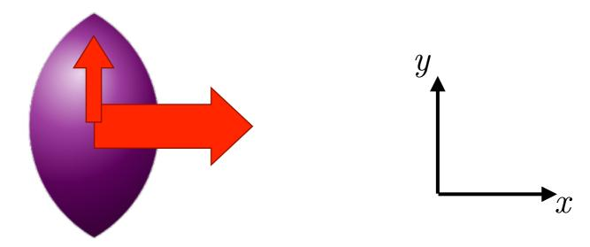
There is matter in the middle, with a given pressure, and vacuum outside: larger pressure gradient along the x-direction than along y. Invoke the Euler eq.:  $[\epsilon(x) + P(x)]u^{\mu}(x)\partial_{\mu}u^{\nu}(x) + \nabla^{\nu}P(x) = 0$
