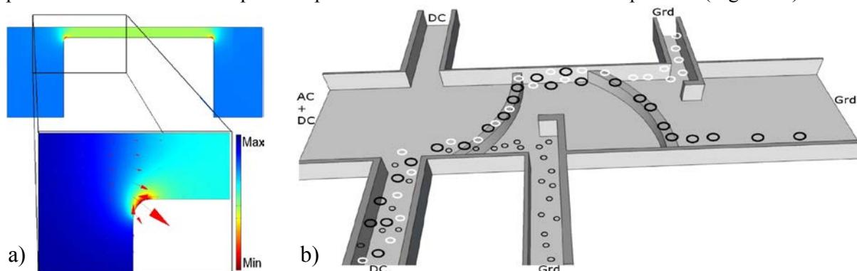
Figure 1: a) Simulation of DEP potential at insulating ridge. b) Sketch of device layout and separation principle. A DNA mixture (circles) was led towards the ridges. Due to different DEP potentials of the DNA species size dependent trajectories appeared at the ridges and resulted iterative separation of the three species.
